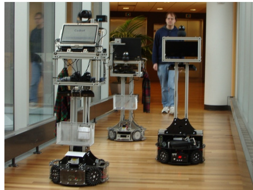
Figure 1: CoBot-1, CoBot-2 and CoBot-4 navigate through the building to deliver items requested by users.
