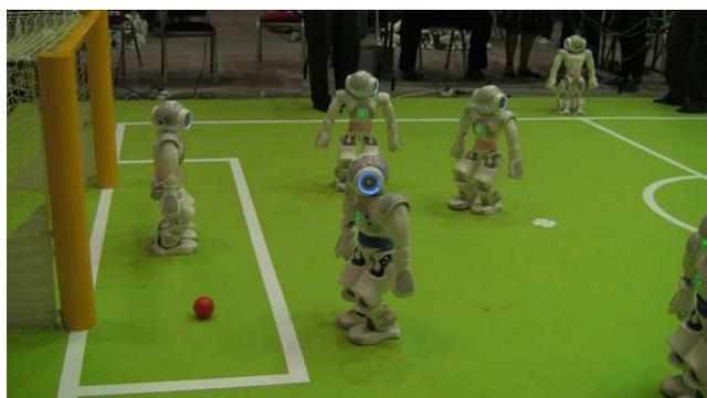
Fig. 1: In the RoboCup SPL, NAO humanoid robots compete at soccer on a 4m X 6m field, with color coded goal posts and field lines which the robots use to localize.
