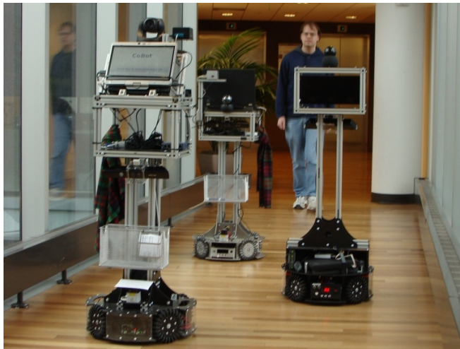
Fig. 1: CoBot-1, CoBot-2 and CoBot-4 navigate through the building to deliver items requested by users.
